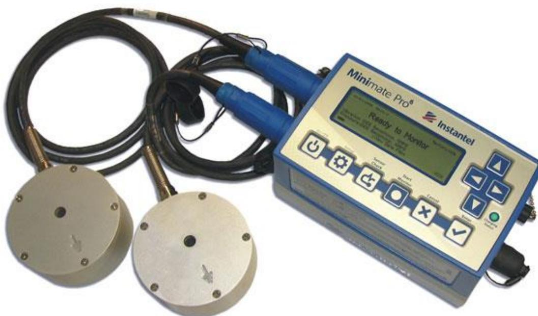
Figura 14 – Sismógrafo InstanTEL® Minimate Pro 6 (InstanTEL, s.d.)
